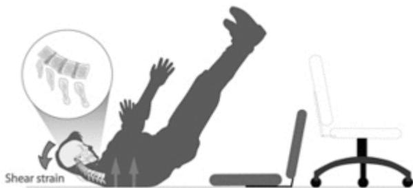
**Figure 1.** This illustration shows the broken chair and the first point of contact with the floor. It also illustrates that shear strain would have resulted as the thoracic spine was abruptly decelerated while the head's inertia carried it rearward relative to the torso. The inset was used to explain the effect of shear on the discs that were claimed to have been injured.
